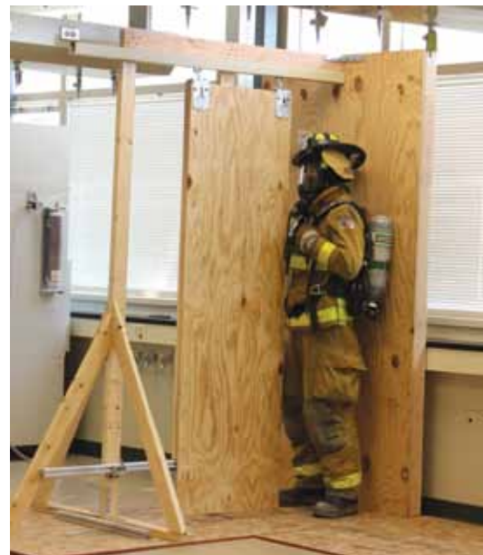
A firefighter with SCBA navigates various space configurations to measure gait, functional balance and other factors.
