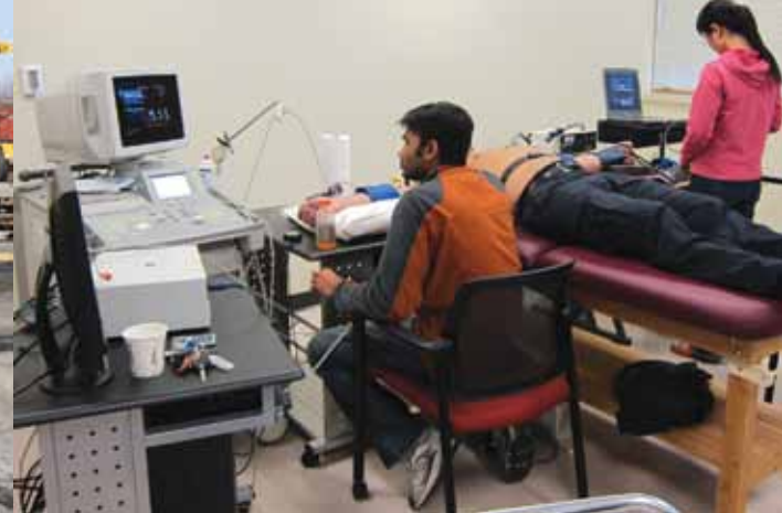
After completing live fire activity, a firefighter returns to the laboratory for detailed cardiac and vascular analysis. The researcher on the left is performing an ultrasound of the brachial artery to measure blood vessel stiffness and flow. The researcher on the right is measuring changes in microvascular reaction. By comparing these factors – and many more – before and after the live fire activity, researchers can learn how the body's cardiovascular system reacts to the stresses of fire fighting.
